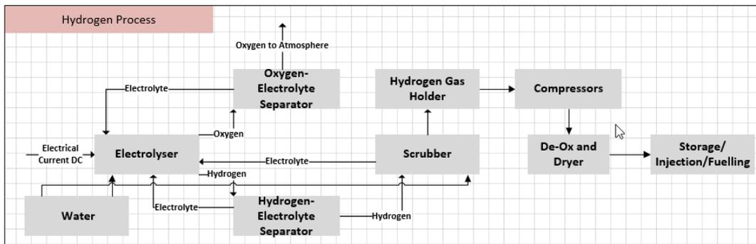
**Figure 4.8 Schematic of the alkaline water electrolysis process**
