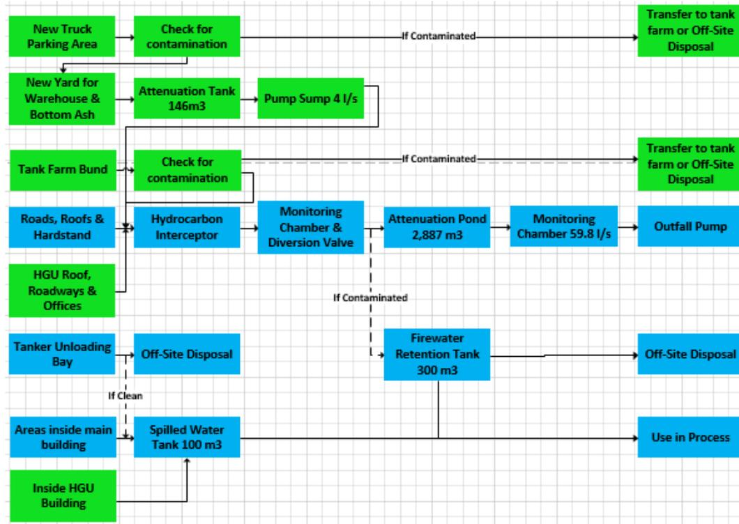
Figure 4.14 Proposed Stormwater Drainage System Flow Diagram.
