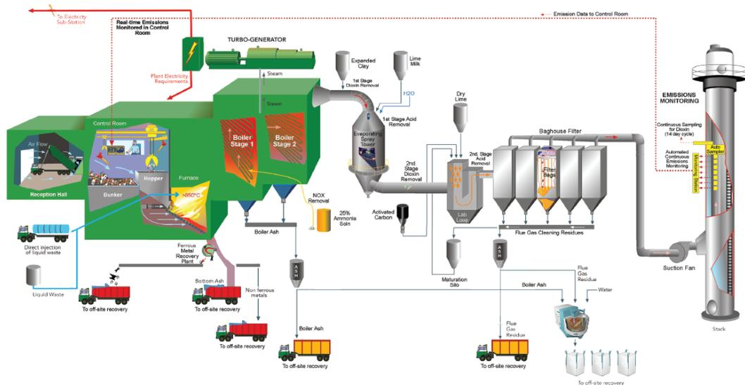
**Figure 4.3 Schematic of the waste to energy process**
