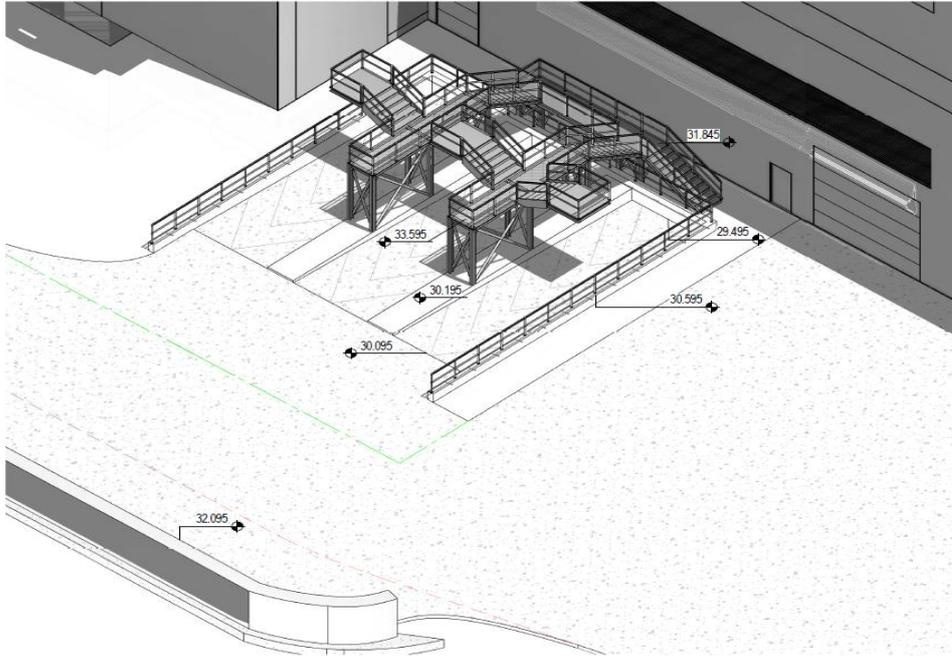
**Figure 4.6 Proposed Upgrade to Existing Tanker Unloading area**
